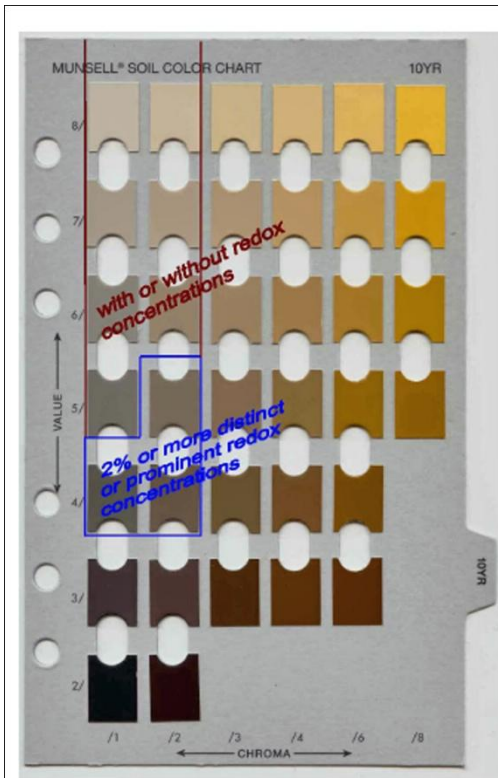
Figure A1. Illustration of values and chromas that require 2 percent or more distinct or prominent redox concentrations and those that do not, for hue 10YR, to meet the definition of a depleted matrix.
